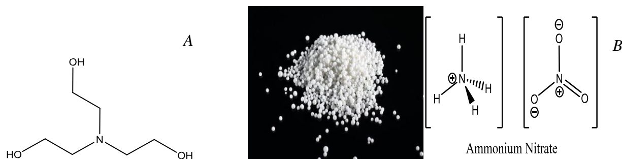
Figure 6. A) Chemical structure of TEA and B) Chemical structure of AN and the pills form
